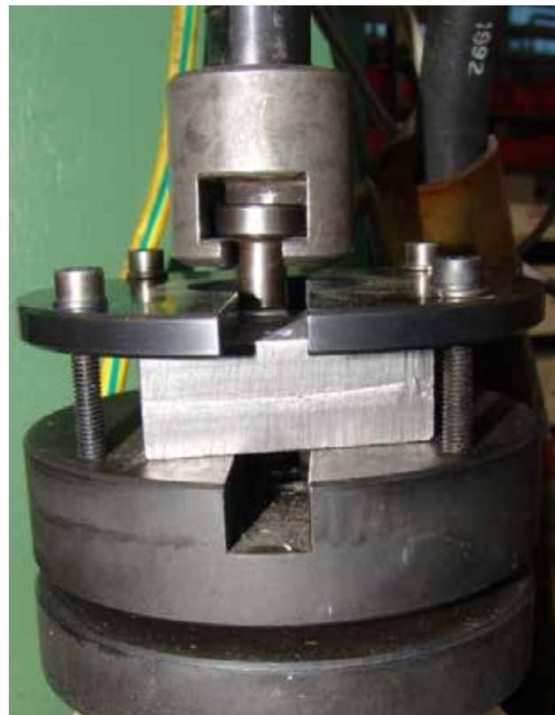
**Figure 5.** Servo-hydraulic test setup for tension fatigue tests
