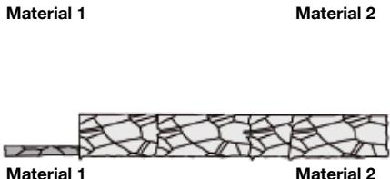
If the surface of the less “noble” material (1) is greater than that of the more “noble” material (2), it will act as a very small cathode and the current density on the “large anodic” less noble material will be very small. Further, this also implies a very low rate of corrosion of the “less noble” material due to electrochemical effects.
