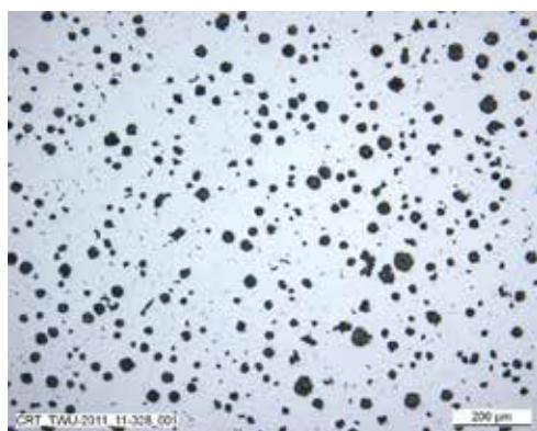
**Figure 3.** Micro section of cast iron EN-GJS-400-18LT:
