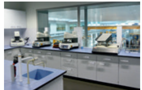
Fig. 23: Metallographic laboratory equipment (grinding and polishing).
